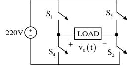
The RMS value of the fundamental component of  $v_o(t)$  in volts is \_\_\_\_\_. Key : 196 to 200
