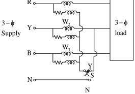
If the switch is connected to Neutral, then each wattmeter will read  $1-\phi$  power.
