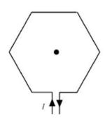
Key: 0.65 to 0.75 Exp: For a finite length conductor B at a point P  $B = \frac{\mu_0 I}{4\pi r} (\cos \alpha_1 + \cos \alpha_2)$
