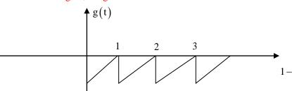
Since this wave form contain hidden half wave symmetry, even harmonics does not exist. Thus coefficient of second harmonic component of Fourier series will be zero.
