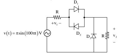
The DC components of voltages  $v_1$  and  $v_2$ , respectively are (A) 0 V and 1 V (B) -0.5 V and 0.5 V (C) 1 V and 0.5 V (D) 1 V and 1 V
